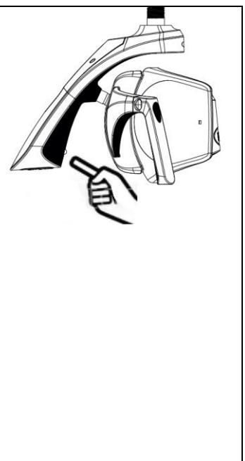
When the Room Lamp is synchronised with the Dental Lamp the blue LED on the Room Lamp is lit steadily. If the LED goes out, this indicates that synchronisation is not active.
