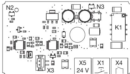
X1 Cleaning button for switch control panel
